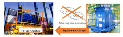
(2) Establishment of a hydrogen supply system for cargo handling machinery Hydrogen is transported from the hydrogen production plant in Chiba Prefecture to Oi Container Terminal using trailers. At the terminal, the hydrogen pressure is increased by using a hydrogen supply unit to fill the RTG tank.
